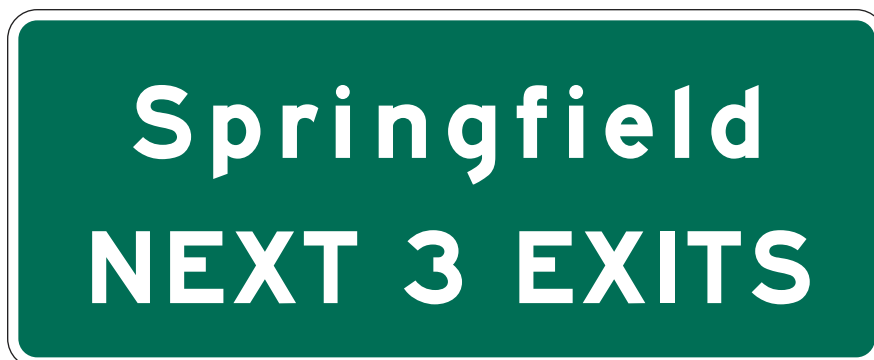
Figure 2E-26. NEXT EXITS Sign
