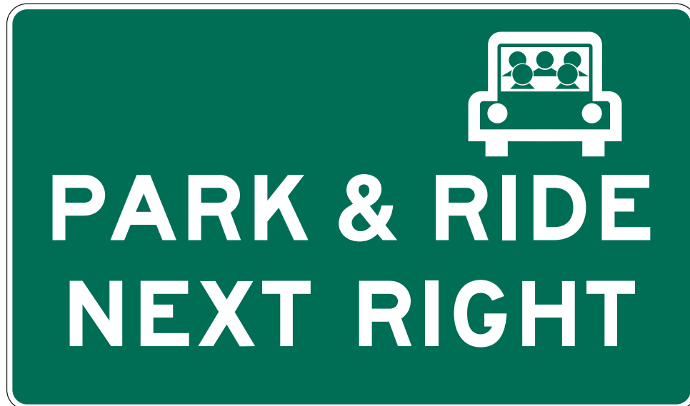
Figure 2E-18. Supplemental Guide Sign for a Park and Ride Facility (Route without Exit Numbering)
