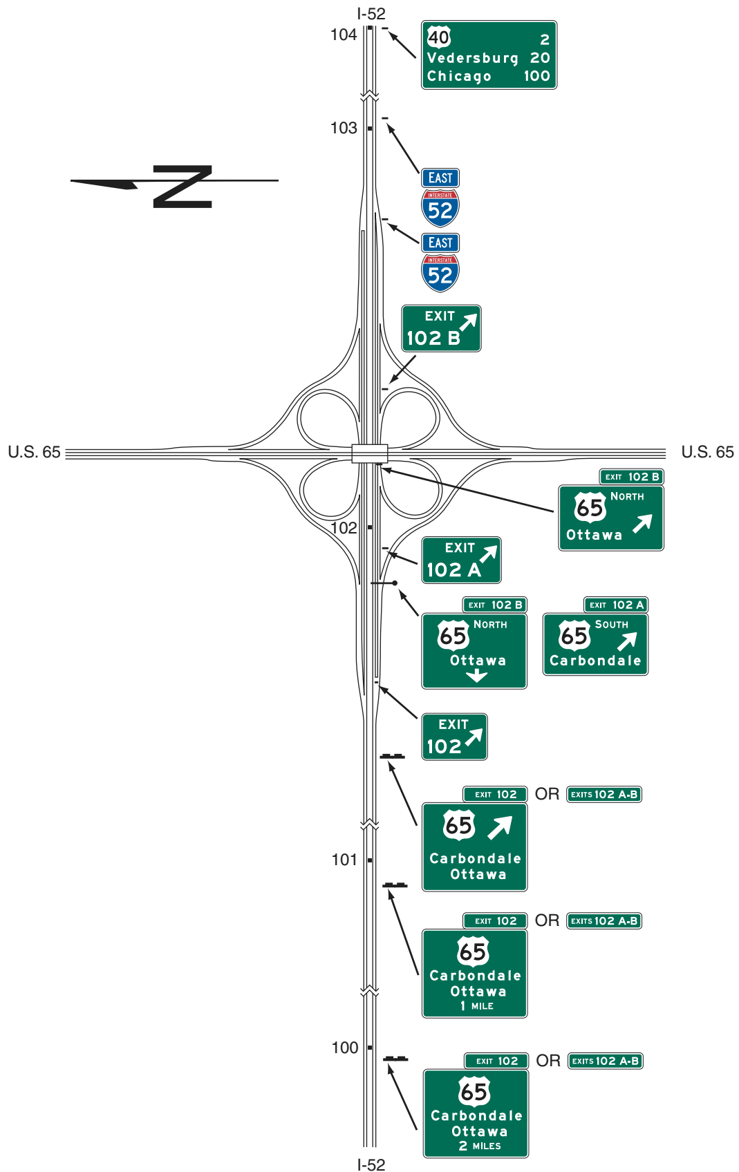
Figure 2E-29. Examples of Guide Signs for Full Cloverleaf Interchange With Collector-Distributor Roadways
