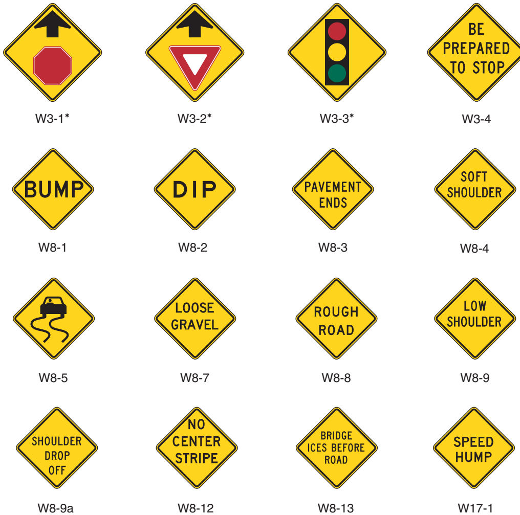
Figure 2C-4. Roadway Condition and Advance Traffic Control Signs
