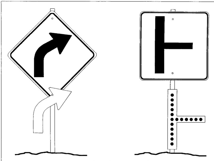
Figure 2. Traffic signs for blackout conditions.
