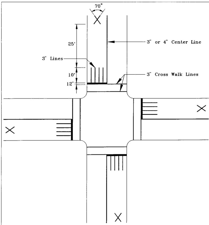
Figure 3. Blackout markings at intersections.
